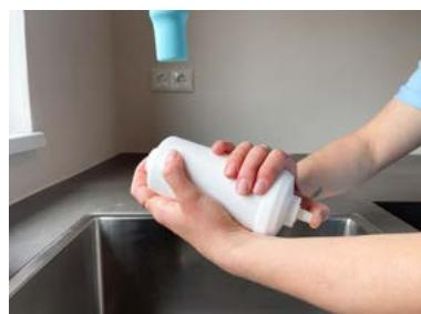
7. Remove the element from the blue primer. Cover both ends of the element with your fingers, or provided blue caps and shake vigorously for 1 minute.
